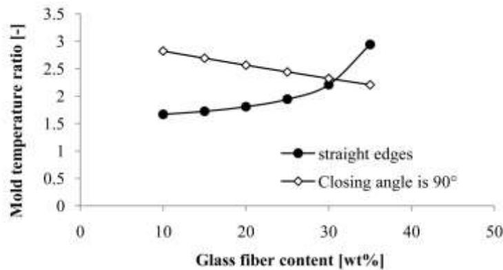
**Figure 7. Required theoretical glass fiber content and mold temperature difference to enable the injection molding of a non-deformed specimen**
