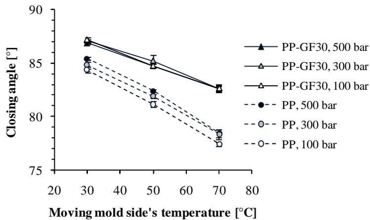
**Figure 4. The influence of the holding pressure on the closing angle as a function of moving mold side's temperature (PP, PP-GF30, the stationary mold side's' temperature is 50°C)**
