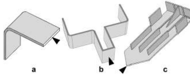
**Figure 1. Specimen geometries with their injection locations for deformation measurements used by a) Jansen et al. [16], b) Ammar et al. [17] c) Mlekusch [22]**
