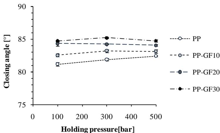
**Figure 5. The effect of holding pressure on the deformation at a relative edge length of 50%**
