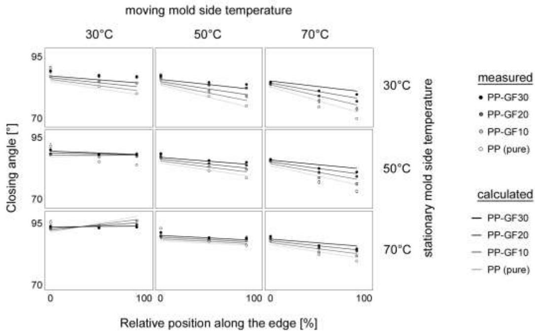
**Figure 6. The effect of glass fiber content and mold temperature on the closing angle as a function of relative edge length**
