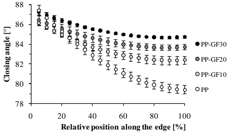
**Figure 3. The effect of glass fiber content on the closing angle as a function of the relative edge length of the specimen (both core and cavity temperatures of 50°C)**
